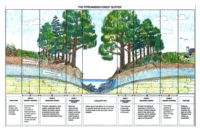
Figure No. 2 – A Riparian Buffer for Protecting a Karst Sinking Stream.
