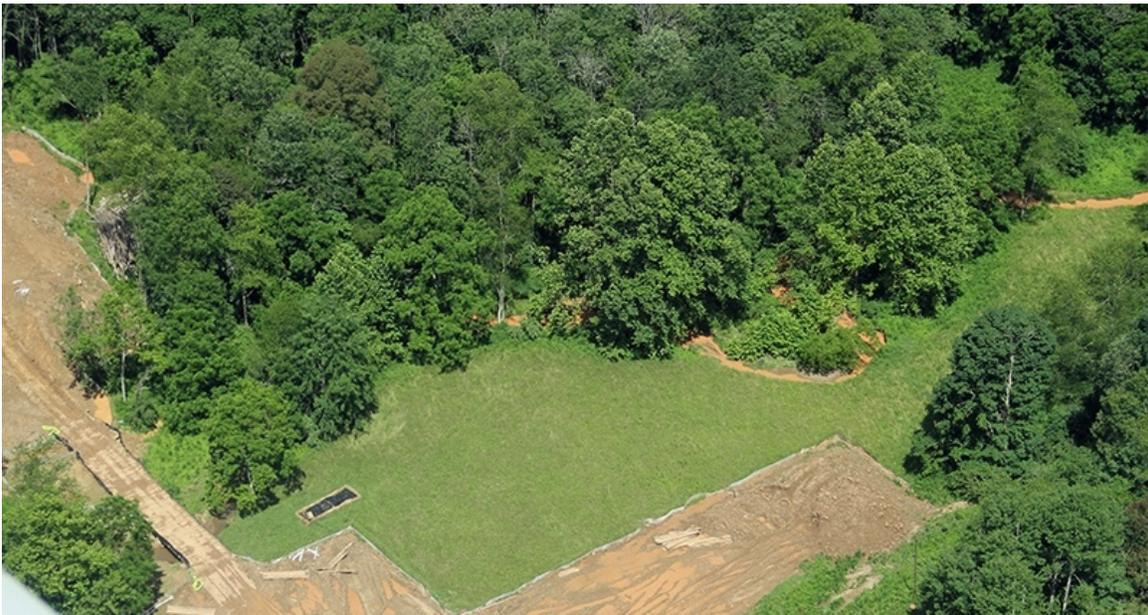
**Stonewall Gathering Pipeline Construction in a Flat Valley with the Stream Crossing Shown in the Lower Left-hand Corner and Heavy Stream Sedimentation Flowing Eastward Towards the Upper Right-hand Corner.**
